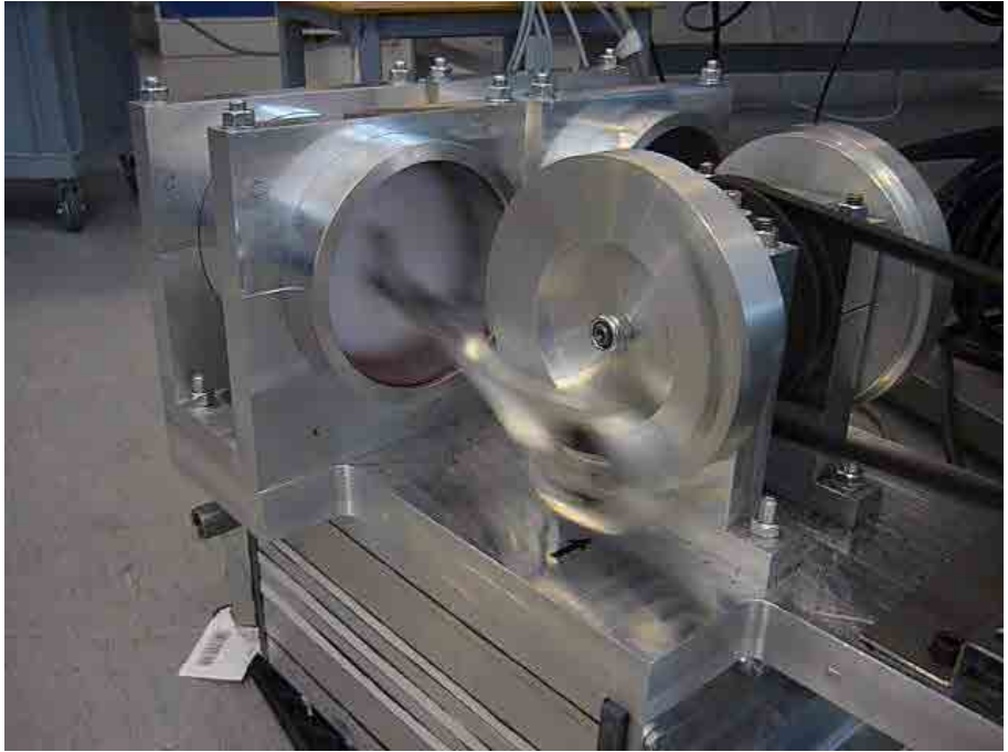
FIGURE 4. Image of experimental setup. The crank shaft is driven by a belt from the electric motor. Cylinders of V_1 and V_2 are mounted on top of heat exchangers and regenerator. First heat exchanger HE_1 , regenerator Rg and second heat exchanger HE_2 are separated by insulation material (white).
