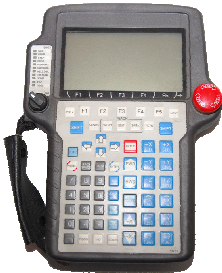
Figure 6.7.1 Control pendant for controlling the movements of the Robotic Arm
