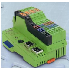
Figure 3.1 A typical PLC with 8 inputs and 4 outputs and Ethernet connection
