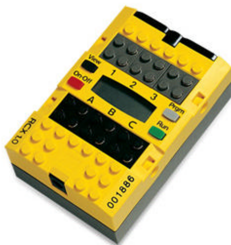
Picture 3. LEGO Mindstorms RCX brick /1/.
