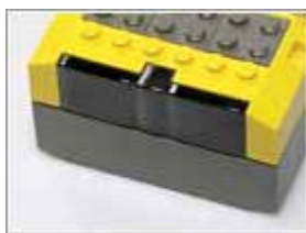
Picture 14. RCX Infrared eye /3/.
