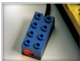
Picture 8. LEGO Light sensor /2/.
