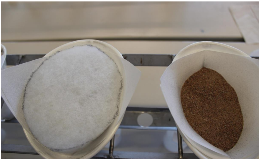
Figure 7. On right using sand filter and on left use of sponge on the top of filter.
