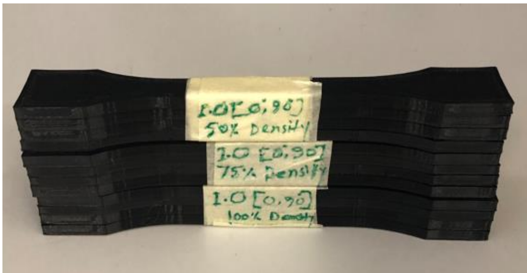
Figure 7. Printed Specimens at different densities and infill orientation (0°, 90°)
