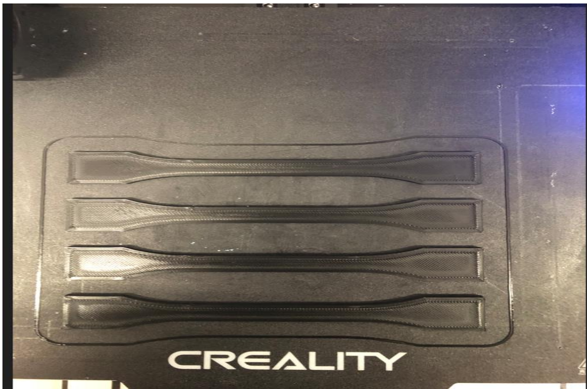
Figure 6. Tensile Test Specimens in Creality Ender-3 Pro 3D Printer
