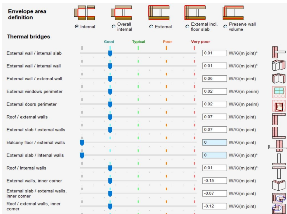
Figure 3. Thermal bridges of the envelope area
