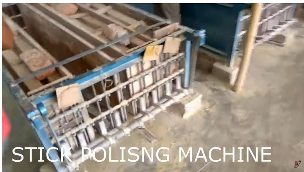
Figure 8: Polishing of Bamboo sticks ( https://www.youtube.com/watch?v=-r9-oz03-g0 )
