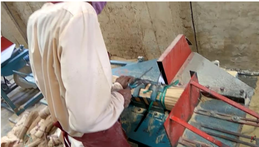
Figure 9: Cutting the round stick bamboo ( https://www.youtube.com/watch?v=-r9-oz03-g0 )
