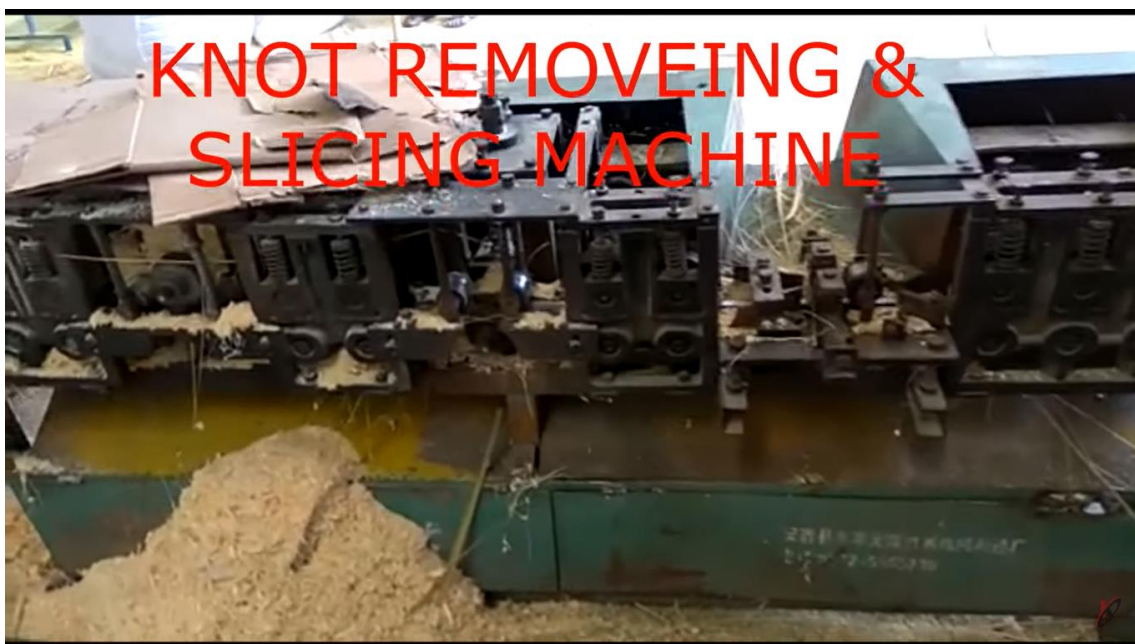
Figure 6: Splicing or slicing of bamboo sticks ( https://www.youtube.com/watch?v=-r9-oz03-g0 ).
