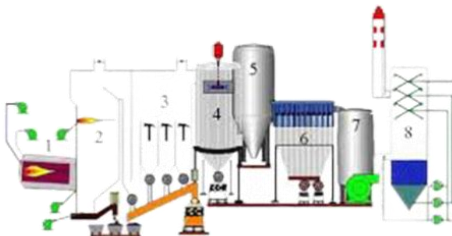
Figure 2: The flow chart of the incineration (Nagy & Kuti 2016,231-237)
