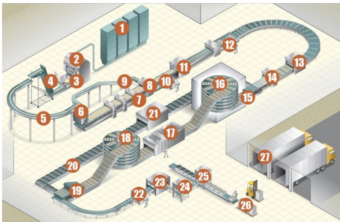
Figure 3. Representation of a 3-dimensional CAD scheme of the Flexco Bakery Layout Design carefully organised arrangement of production zones, manipulation of the machinery placement effective use of space, and customer flows management (Industrial Baking Map Bread, 2024).
