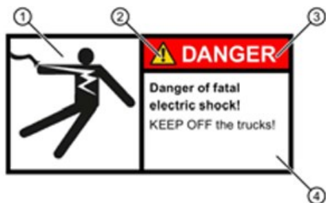
Figur 37: Exempel på varningssymbol enligt definitioner i ANSI Z535.4. (Industrial Control Panels and Electrical Equipment of Industrial Machinery for North America, 2014).
