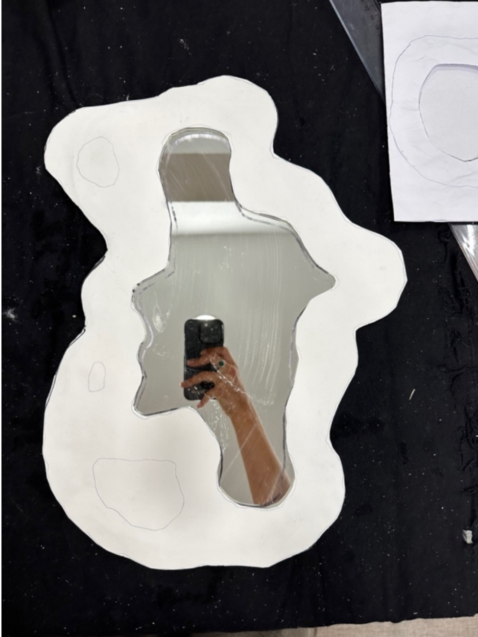
Figure 16 Using a paper template of the foam glass frame for shaping the mirror for the final piece
