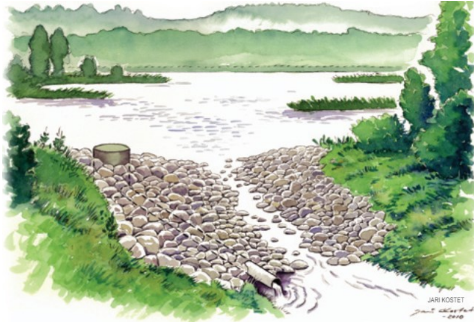
Figure 5. A bottom overflow dam (Alhanen et al. 2015, 33.).
