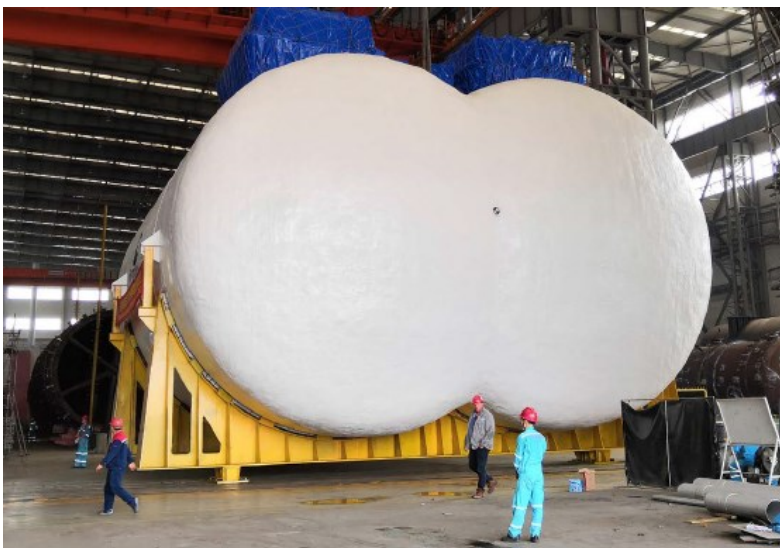
Figure 2. PUF-insulated bilobe tank (Wärtsilä Internal Document, 2018).
