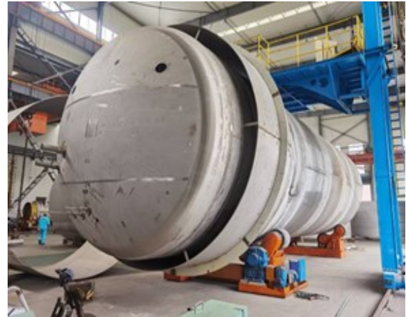
Figure 5. Dish end installed (Wärtsilä 2022).
