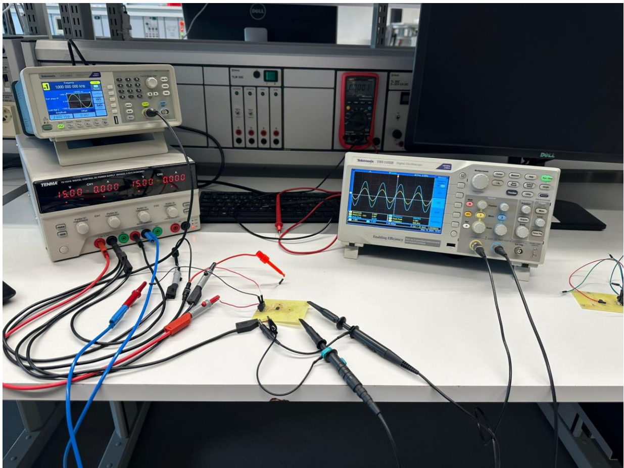
Figure 32. The setup of the tested op-amp circuit
