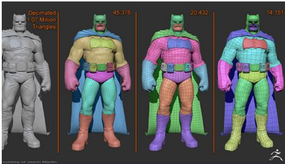
Figure 4. Example of polygon reduction: from 1.07 million triangles to 14 151 (Lesterbanks 2013)
