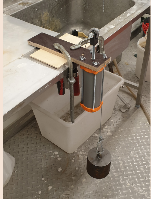
Image 13. Testing of the weight driven system.
