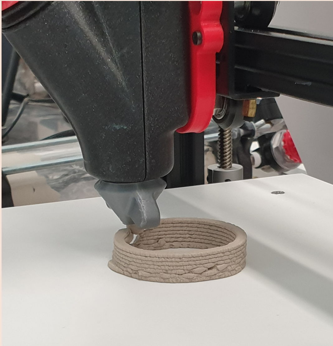
Image 44. The first test print was really promising. The layers look good. With little optimisation to the settings proper printing will be possible.
