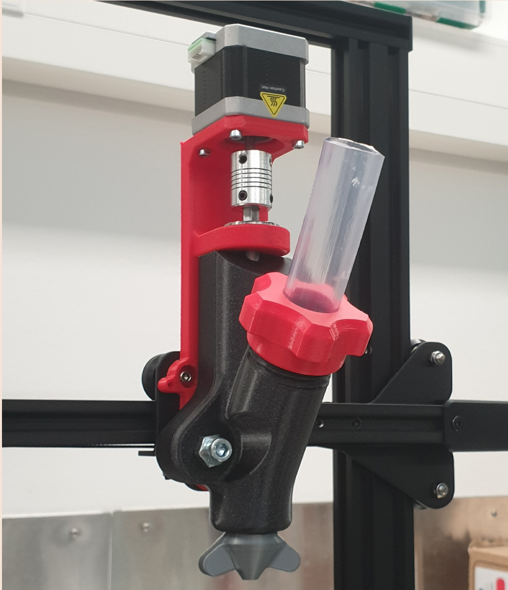
Image 40. The extruder attached to the 3D printer looks clean and professional. The nozzle is also 3D printed allowing customized nozzle shapes.
