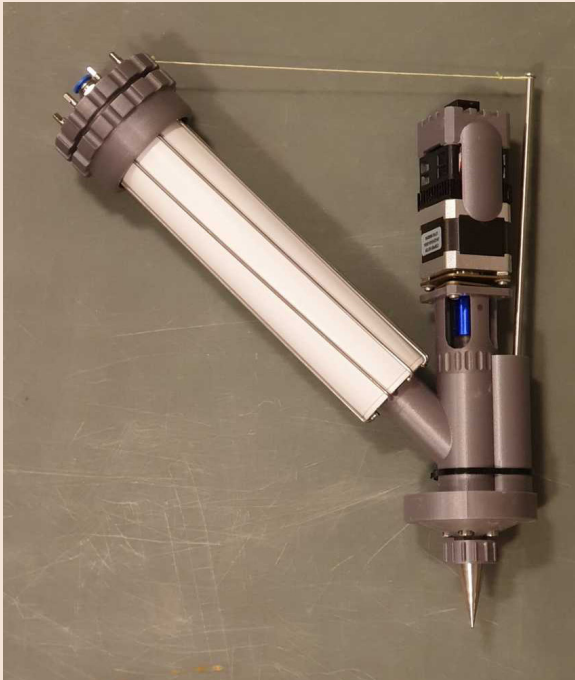
Image 7. A extruder utilizing empty silicon gun cartridges and bicycle spokes.
