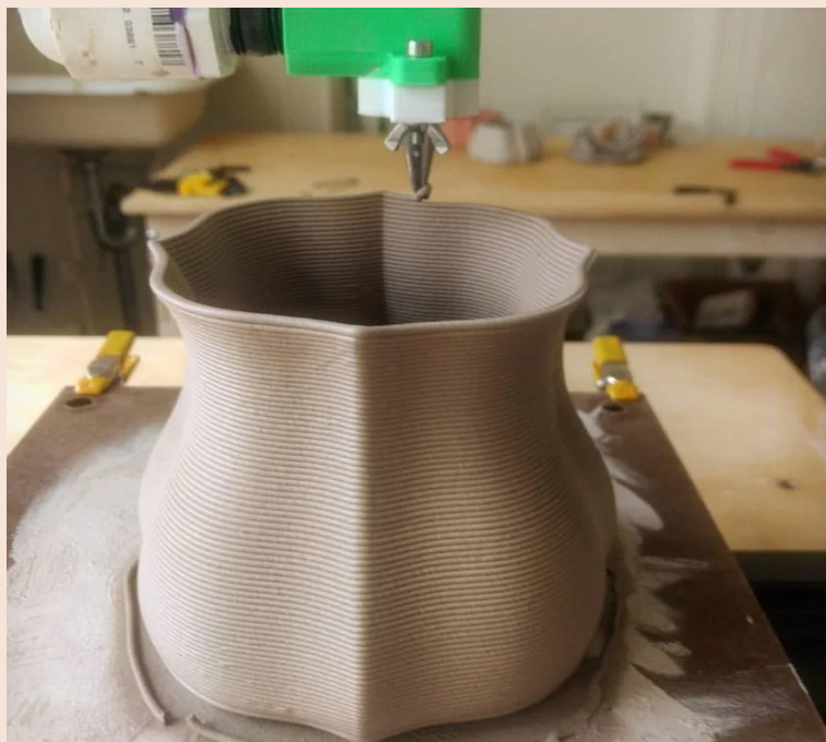
Image 3. Clay 3D printing in progress, posted on Thingiverse by the user Lauhaus.
