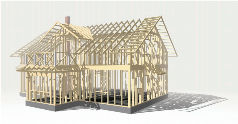
PICTURE 1. In Timperi timber frame system, each wooden part is planned separately before machining and construction.
