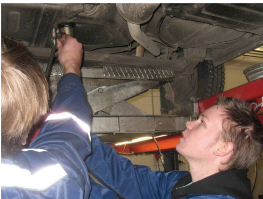
PICTURE 2. Students draining the fuel system of a car to be scrapped. Photo by Markku Ikonen.
