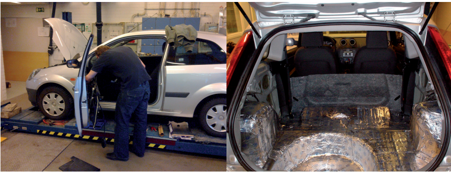
PICTURE 2. Insulating the front door (left) and the back of the car (right). Photos by Pekka Nousiainen.
