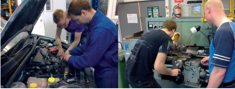
PICTURE 3. Installing boost system pipes (left), peeling connector housing (right). Photos by Pekka Nousiainen.
