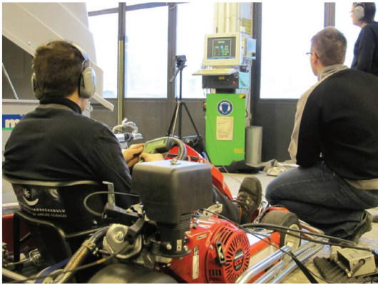
PICTURE 5. Students testing their go-kart car on a chassis dynamometer. Photo by Markku Ikonen.
