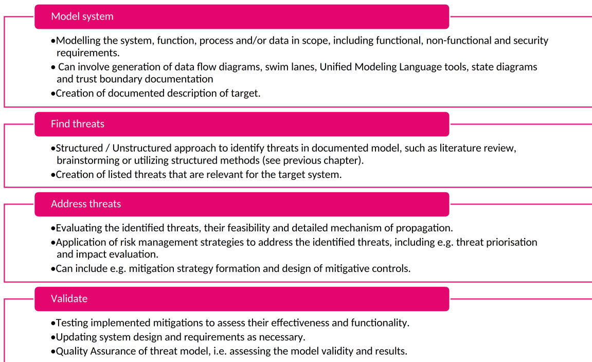
Figure 3: Process of threat modeling (Shostack, Chapter Introduction, 2014, p. 28-30, 44-52, 59-60 & 123-124)
