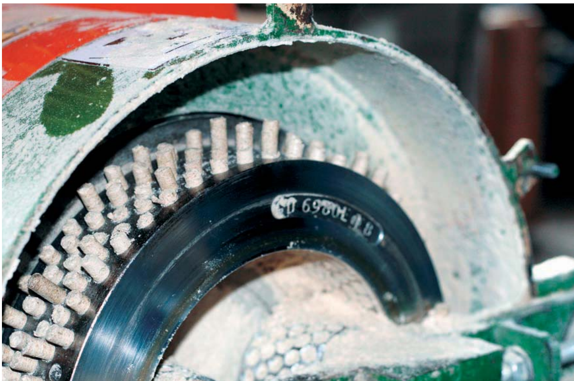
Experimental Common Reed pelletizing on the equipment of Biottori Oy in Jämijärvi. It is possible to press Common Reed into pellets even with small-scale pelletizing machines. When chopped short enough the Common Reed, the right adjustments and a pinch of for instance Turnip Rape pressing waste guarantee a first-class pellet. Photo: Sami Lyytinen.
