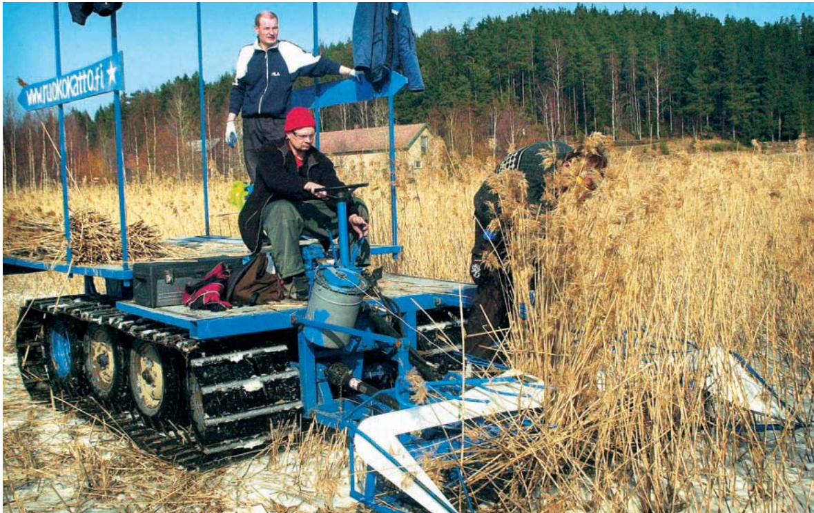
Continuous track machines have a low surface pressure which is a definite help in damp and soft-bottomed reed beds. The thresher in the picture is small and narrow enough to fit onto a trailer which makes it quick and easy to transport on highways. Photo: Pekka Poutanen.
