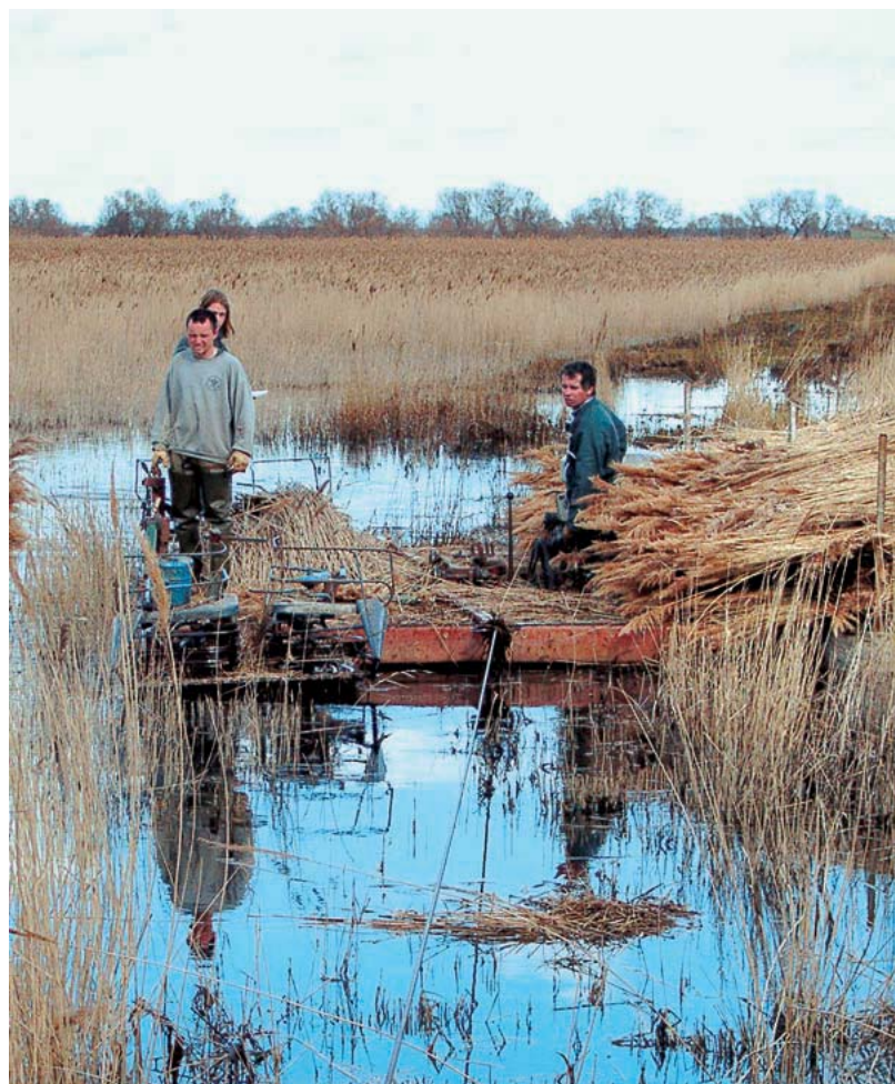
In southern France, reed is collected for building use also from a pontoon moving between two points with the help of a wire. This does not upset the water bottom and stops the bottom nutrients from dissolving into the water. Photo: Brigitte Poulin.
