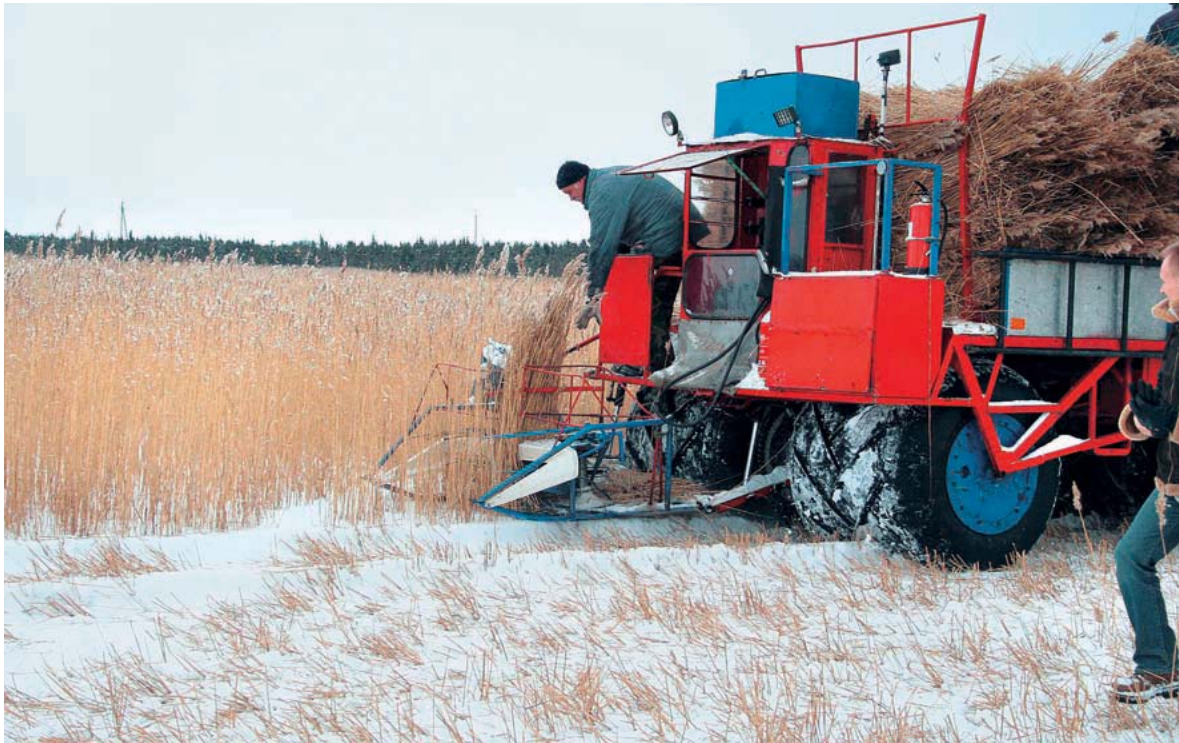
The wide-tyred Seiga was originally designed for rice farming, but it is commonly used for harvesting reed beds in different parts of Europe. In the picture you can see an demonstration of harvesting reed with a Seiga in Halikonlahti, March 2006. Photo: Eija Hagelberg.
