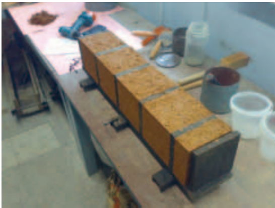
Picture 4: Compressive strength specimens after preparation. Photos: K. Karja and D. Mesteljainen.
