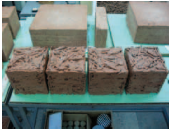
Picture 4: Compressive strength specimens after preparation. Photos: K. Karja and D. Mesteljainen.
