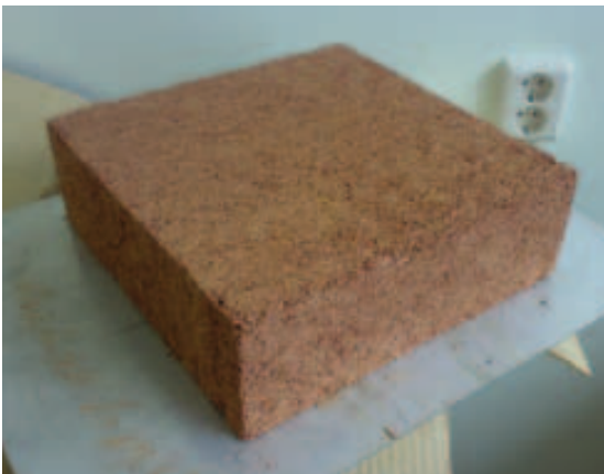
Picture 5: Thermal conductivity specimens after preparation. Photos: D. Mesteljainen and K. Karja.
