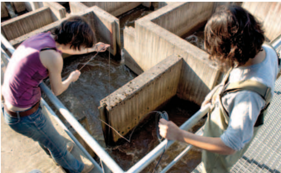
Marianne Decoster-Taivalkoski and Alejandro Montes de Oca are installing the hydrophones in the fish ladder at Halistenkoski, Koroinen. Photo: Thomas Söderström.
