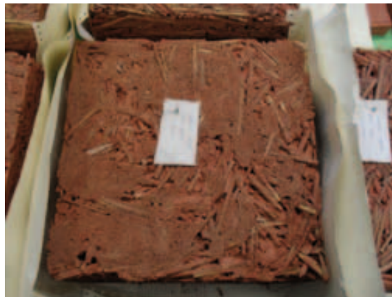
Picture 5: Thermal conductivity specimens after preparation. Photos: D. Mesteljainen and K. Karja.
