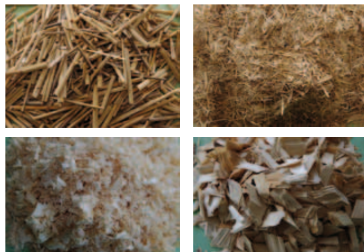
Picture 3: Light additives such as chopped reed, flax shives, wood shavings and chips were added to lightweight clay blocks to increase thermal properties. Photos: Kristina Akermann.
