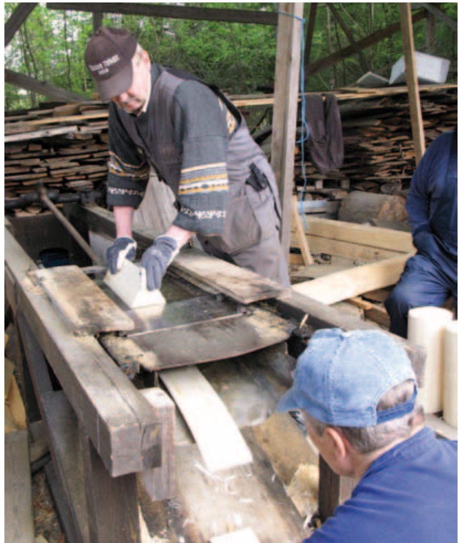
Planing shingles in Rahkio during the spring of 2010. Blade planes shingles from the wood leaving a triangular log.
