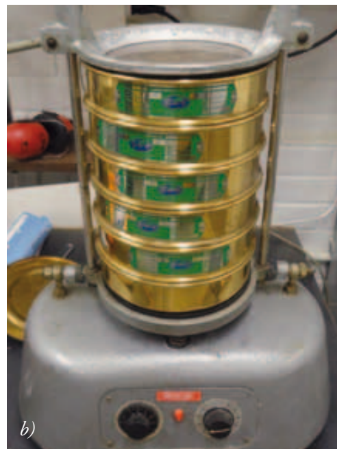
Figure 6: Preparation of the bark samples for the chemical analyses: a) grinding, b) sieving, c) flotation.
