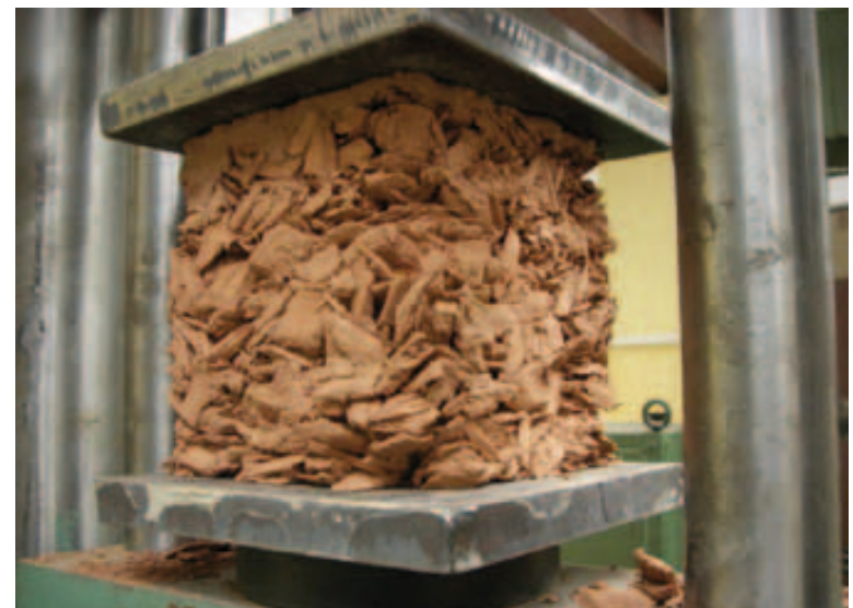
Picture 6: Centrally placed specimen between the two platens of the compression testing machine. Photos: D. Mesteläinen and K.Karja.
