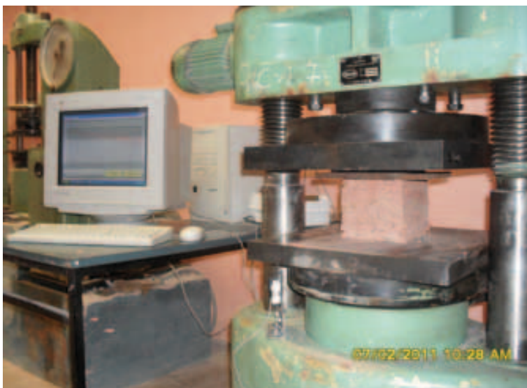
Picture 6: Centrally placed specimen between the two platens of the compression testing machine. Photos: D. Mesteläinen and K.Karja.
