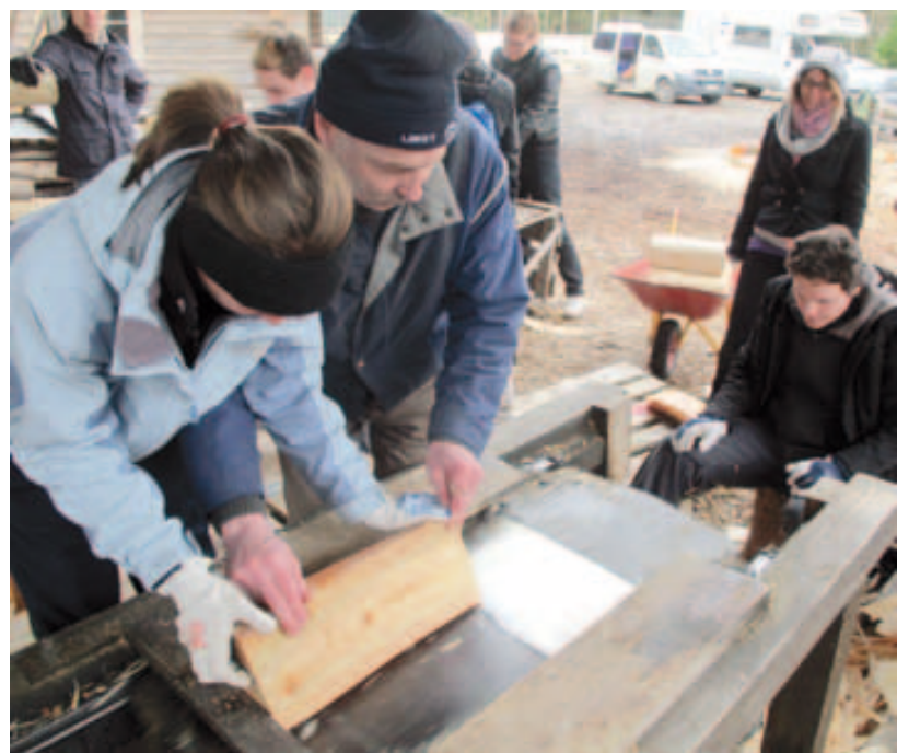
Olavi Mäkinen guiding Anna Pichetto Fratin on how to make thin shingles.
