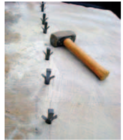
Photo 2: Splitting granite using wedges – ( www.wikipedia.org 2012).
