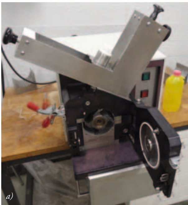
Figure 6: Preparation of the bark samples for the chemical analyses: a) grinding, b) sieving, c) flotation.
