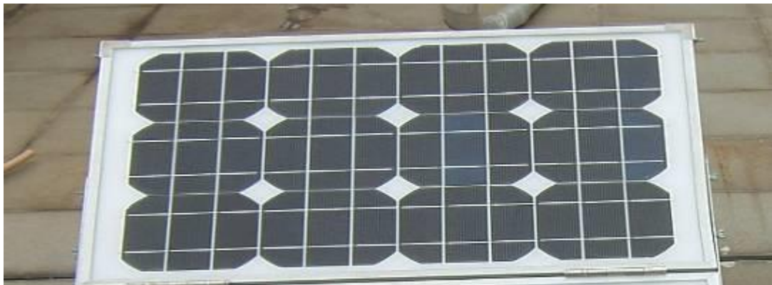
Figure 3. Monocrystalline silicon solar energy cell board (Baidu 2014)
