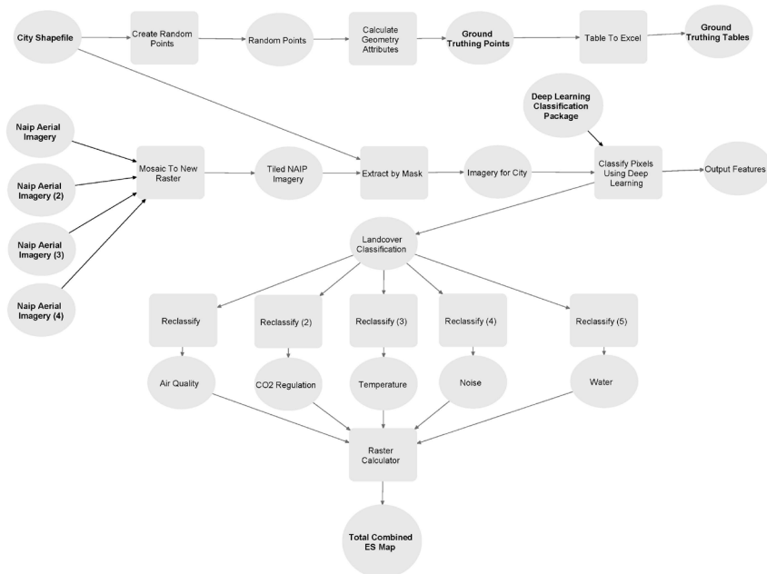
Figure 2. Model builder in ArcGIS Pro for the geospatial methodology in this study
