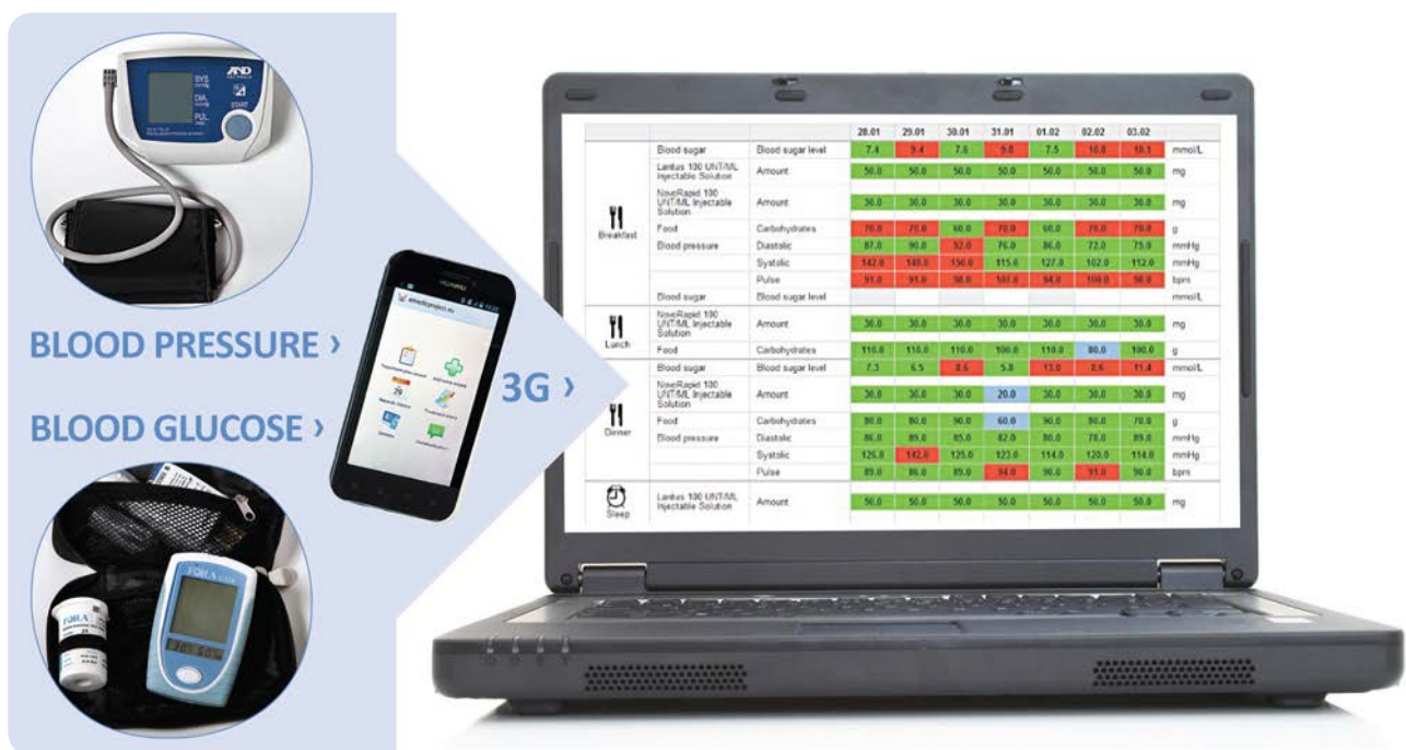
The patient performs blood glucose and blood pressure measurements as usual. Measuring devices are connected via Bluetooth with the Android smartphone which transmits the information to the PHRbox. In the database, the data is available to the patient and to the health care personnel.
