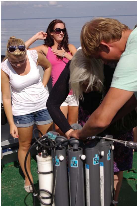
FIGURE 2. Students observing the set-up of the CTD rosette measuring device. Photo: Karin Ojamäe.
