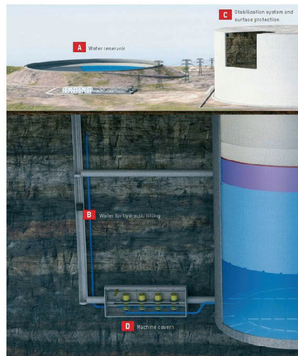
Figure 48. Gravity Storage by Heindl: (A) water reservoir, (B) water for hydraulic lifting, (C) stabilization system and surface protection, (D) machine cavern (Illustration with permission of Gravity Storage GmbH, www.gravity-storage.com )
