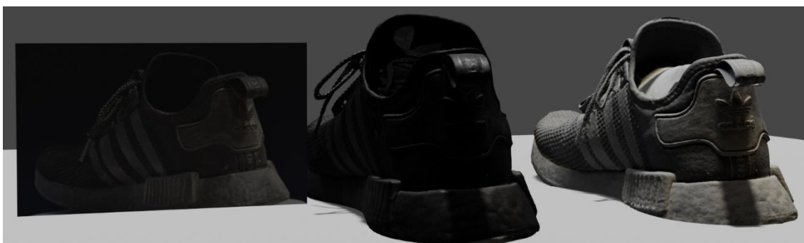
Figure 23. From left to right: original object, digital camera photogrammetry and smartphone photogrammetry.
