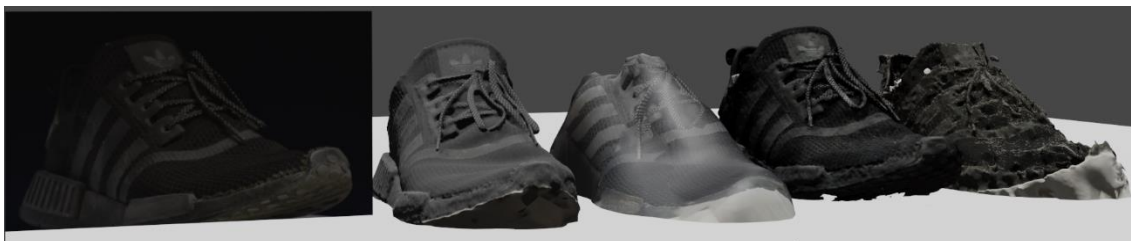
Figure 20. From left to right: original object, smartphone photogrammetry, LiDAR, NeRF and digital camera photogrammetry.
