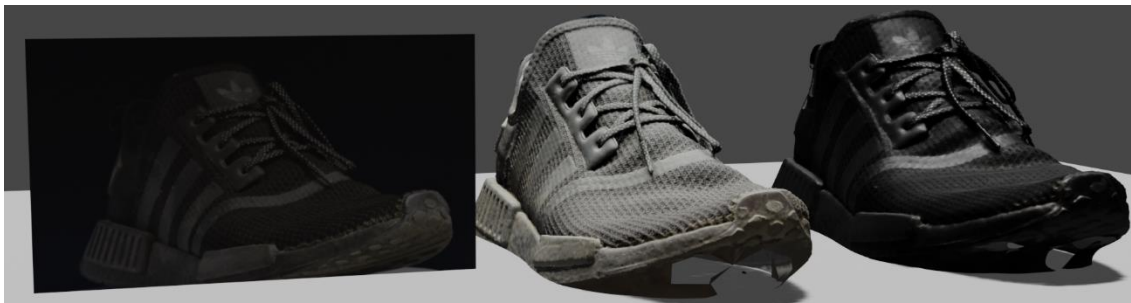
Figure 22. From left to right: original object, smartphone photogrammetry and digital camera photogrammetry.
