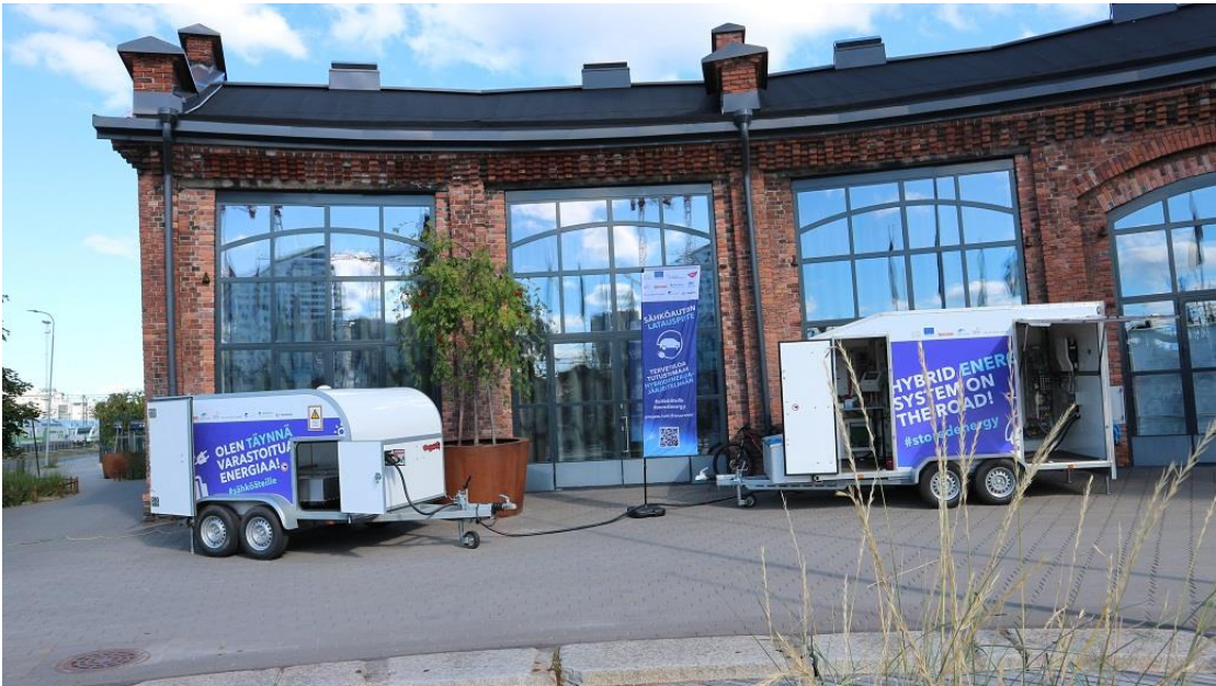
Figure 1. Mobile hybrid energy system built in two trailers. The left trailer includes energy storage system, and the right one encloses power electronics system and high power charging station for electric vehicles. Technically versatile system offers excellent open innovation ecosystem for modern electric drives of smart energy transition. [3]
