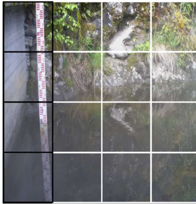
Figure 10. The grid cells with black outlines are cells that are responsible for the localization and prediction of the staff gauge object.
