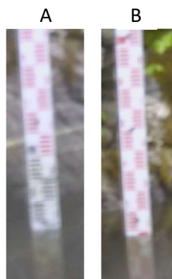
Figure 35. Image A is covered by a haze while image B is out of focus.
