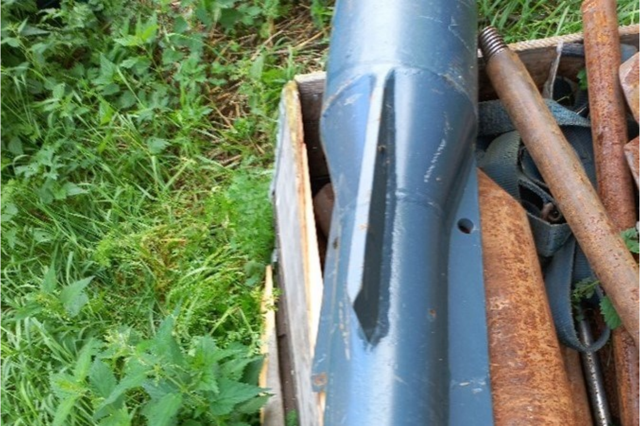
IMAGE 3. The blade of the used pipe splitter [5].
