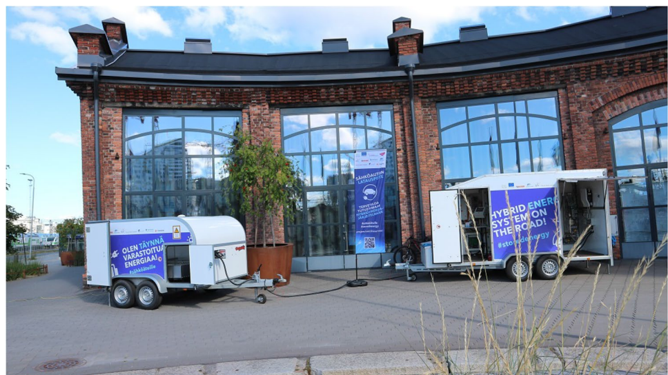
Fig. 1 Mobile hybrid energy system built in two trailers. The left trailer includes energy storage system, and the right one encloses power electronics system and high power charging station for electric vehicles
