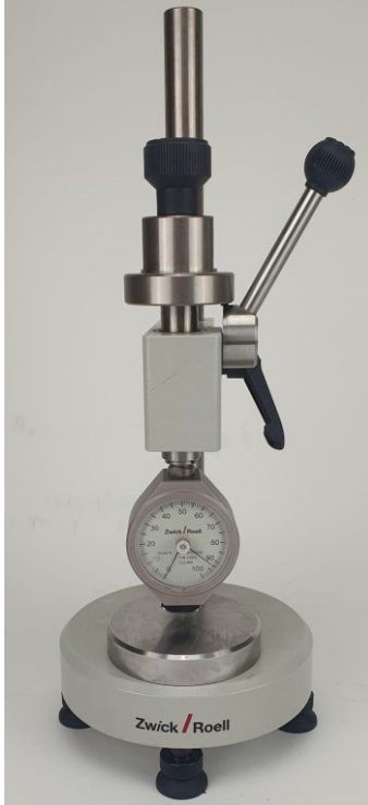
Figure 12. Zwick Roell Shore A with testing stand.
