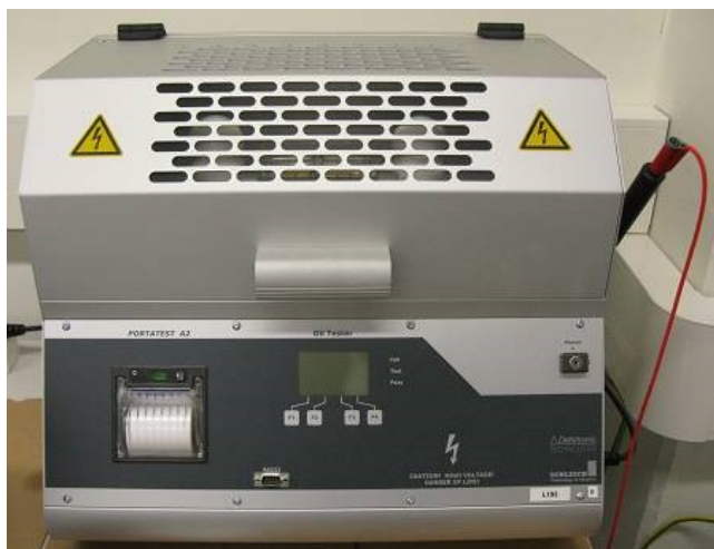
Figure 13. High voltage test device Schleich Portatest A2.
