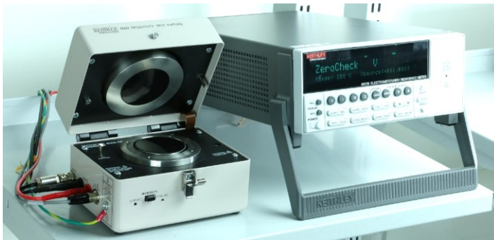
Figure 15. Keithley 6517 B Electrometer and Keithley resistivity test fixture 8009.
