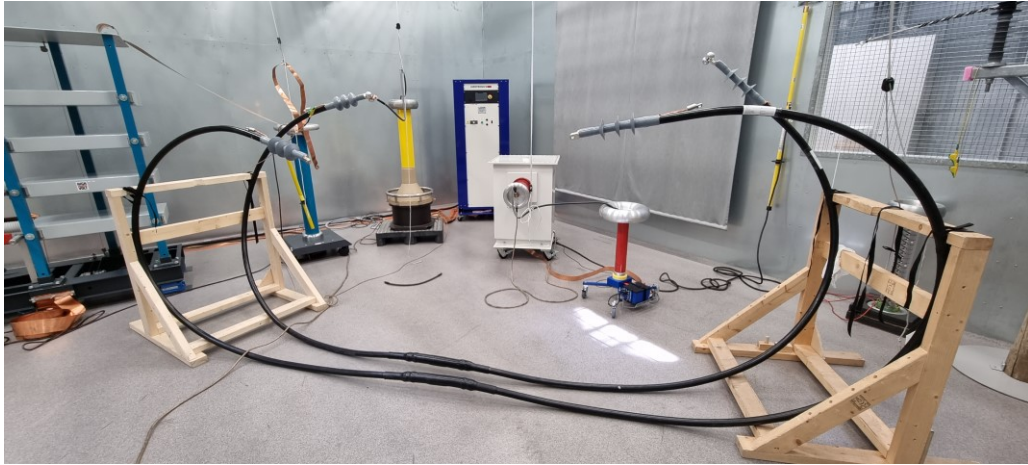
Figure 16. AC voltage dry test set up.
