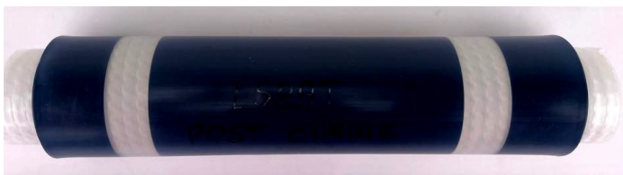
Figure 23. CSJM16 sample for visual and shrinkage examination.
