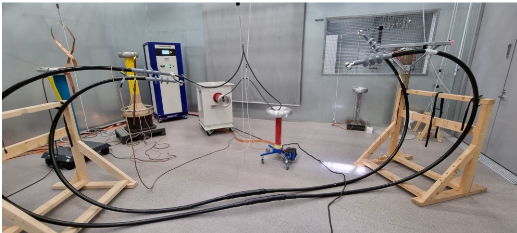
Figure 17. Partial discharge test set up.
