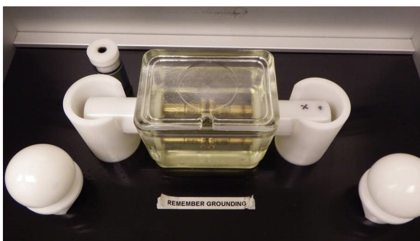
Figure 14. Test cell of the High voltage test device Schleich Portatest A2.
