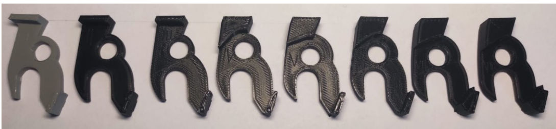
Figure 35. Rapid Prototyping of the notch for the derailleur. (Author's own).
