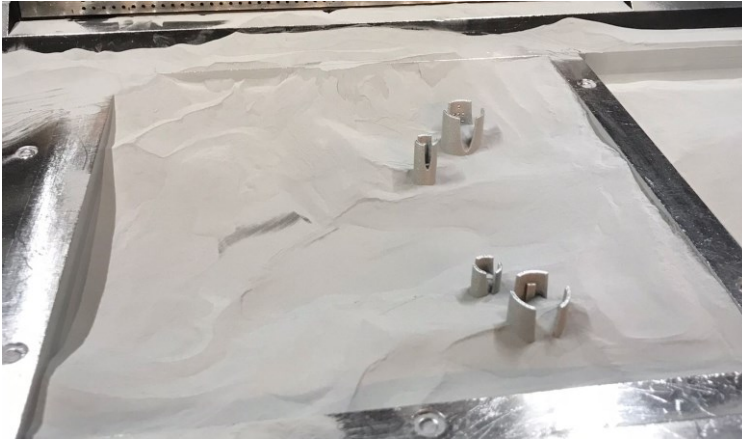
Figure 116. Baseplate covered in metal powder. (Author's own).
