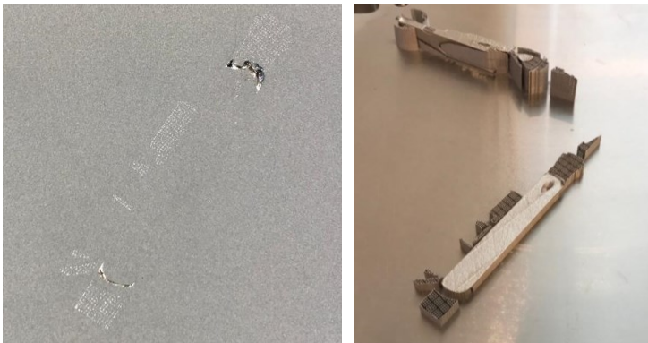
Figure 123. Metal printing error on the left and aborted printing result on the right. (Author's own).
