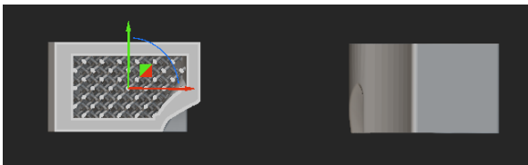
Figure 41. Section for the merge and infill for the auxiliar part (Source: Author's own).
