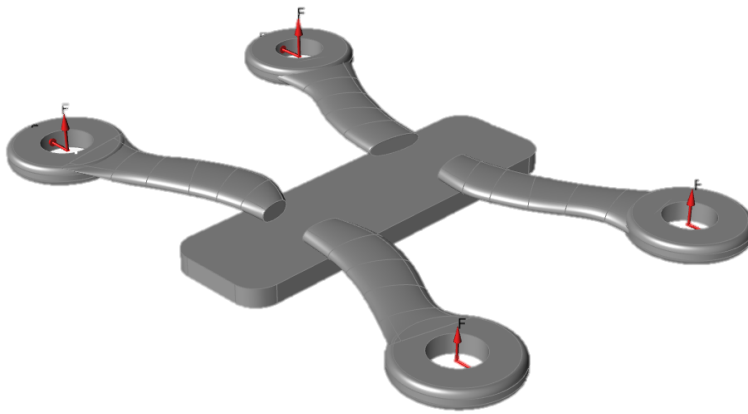
Figure 32. Fit of the optimized part (Source: Author's own).
