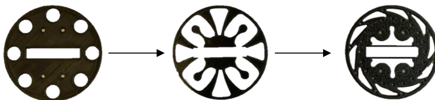
Figure 80. The design evolution of the top disc (Source: Author's own).
