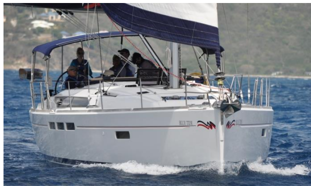
Figure 8. Ship which uses a furler for reefing and unrolling the sail (Source: www.offshoresailing.com ).
