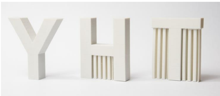
Figure 7. Examples of support generation structures (Source: https://www.hubs.com/ ).
