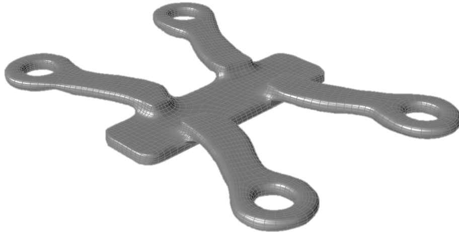
Figure 35. Topology optimization for the cover (Source: Author's own).
