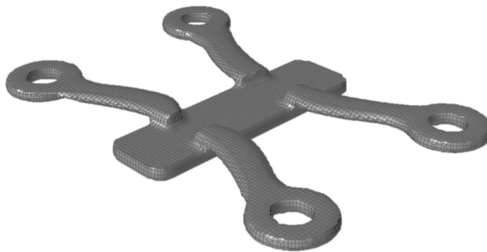
Figure 33. Straightening of the optimized part (Source: Author's own).
