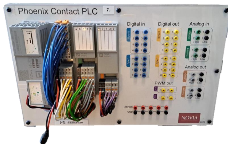
Figure 5: PLC Phoenix contact AXCF. (Source: Author's own)
