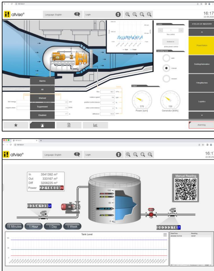
Figure 1: a) b) SCADA example with atvise. (Source: https://www.teslakontrol.com )
