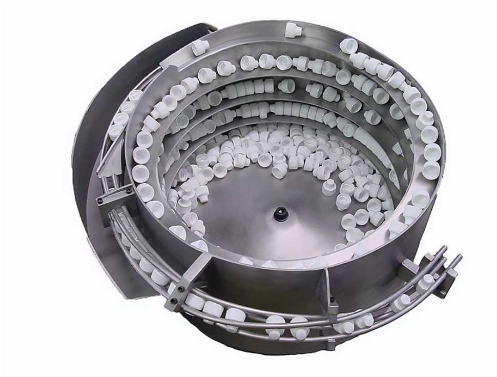
Figure 1- Example of feeding bowl (Source: www.autodev.com )
