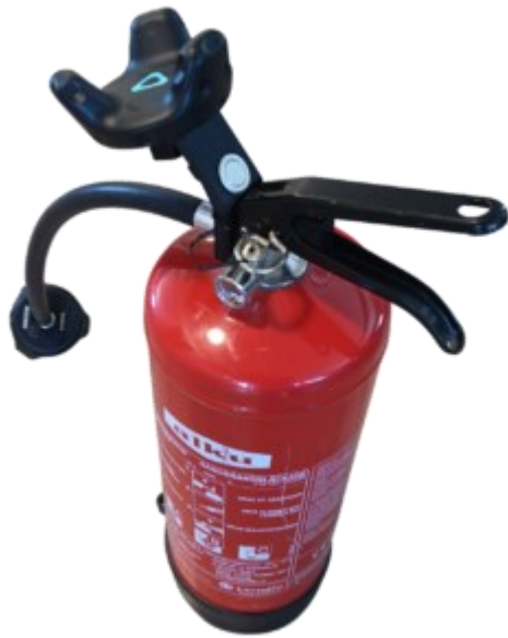
Figure 6. Fire Extinguisher Controller.
