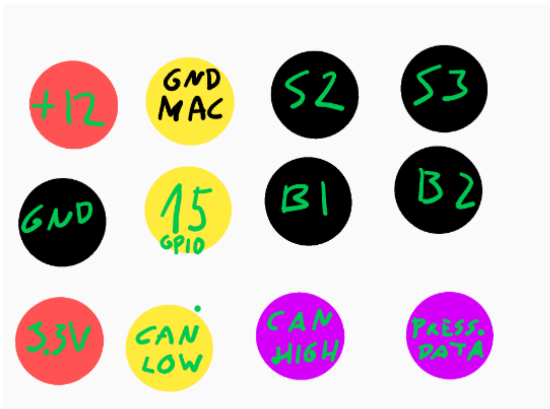
Figure 39. Boost controller's connector pinout with wire colors (front view)
