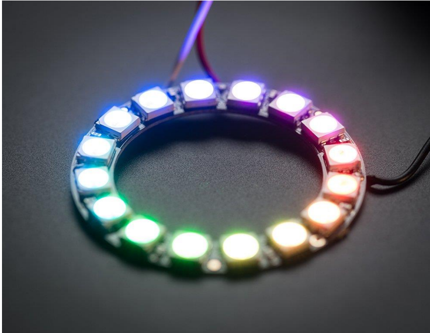
Figure 14. Neopixel Led ring that was used in the project [12].
