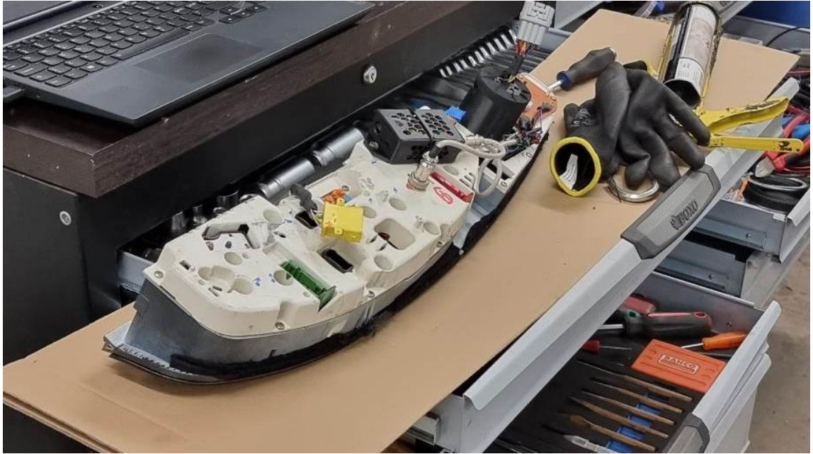
Figure 41. The cars instrument cluster the first prototype was installed
