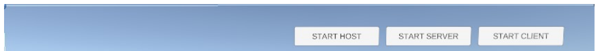
Figure 28. Implementation of network options in the user interface In the script, these buttons need to be referenced and listened to trigger the function StartHost() , StartClient() and StartServer() (Figure 29).
