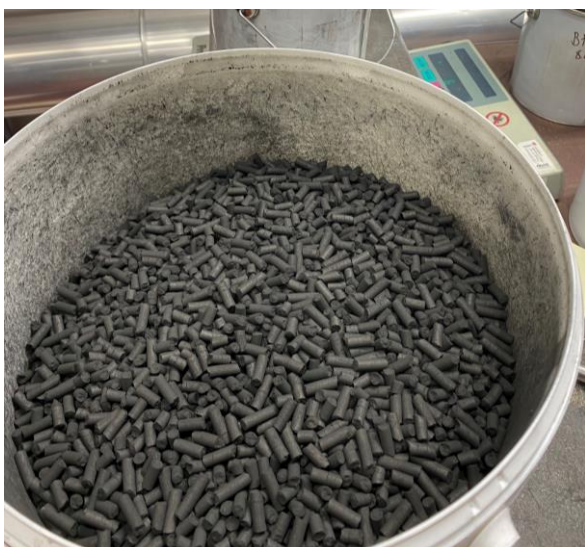
Figure 16. Biochar pellets. BCFB 22/04 -test run's hot filter dust that is pelletized in Germany by an EIFER partner. About 10 % corn starch as a binder.
