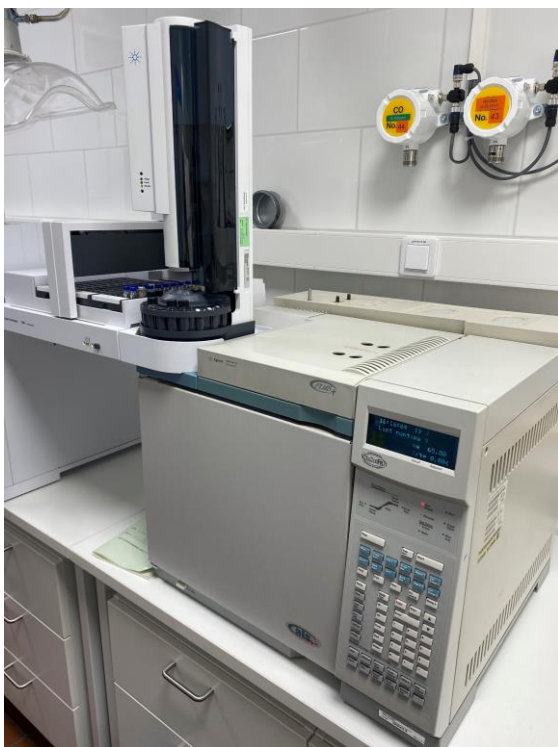
Figure 11. The gas chromatograph (Agilent 6890N) with FID to analyze polycyclic aromatic hydrocarbons (PAH) compounds.
