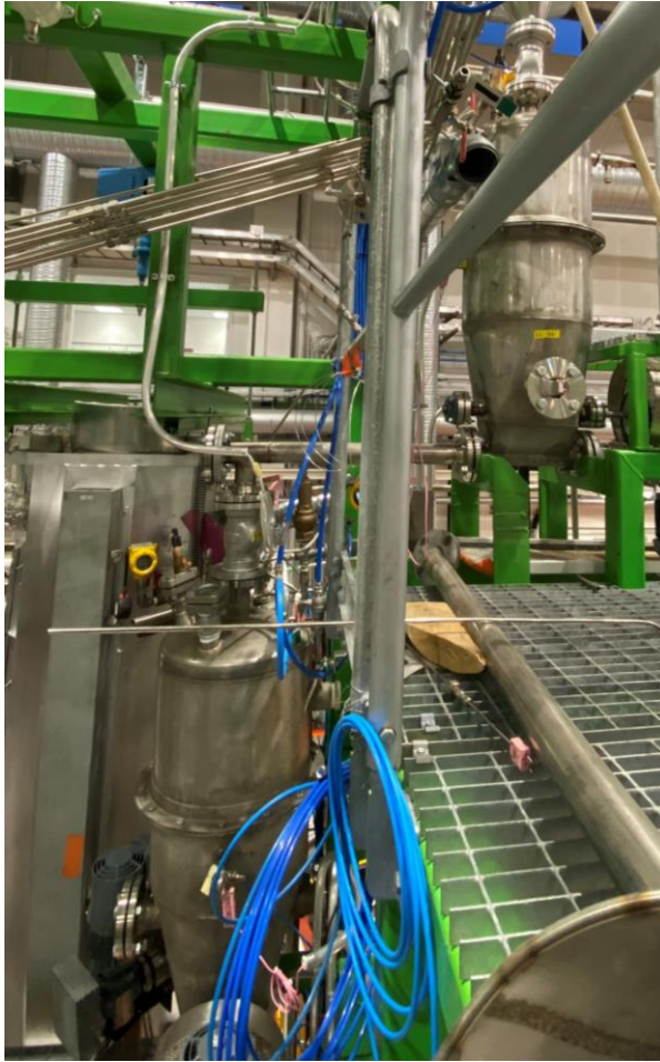
Figure 6. The solid recovered fuel tanks. The filling tank is the upper tank, and the feed tank is the lower tank.
