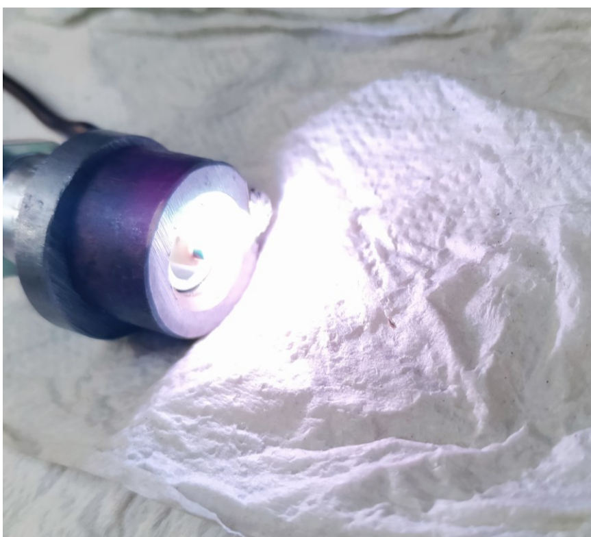
Figure 36. Plasma discharge in air at 295.15 K, 56 \mu\text{F} discharge capacitor charged to 354 VDC, discharge energy before losses 3.5 J.
