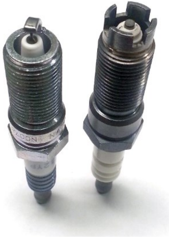
Figure 16. Conventional spark plug (left) and low-energy transient plasma spark plug (right) (60, p. 2).
