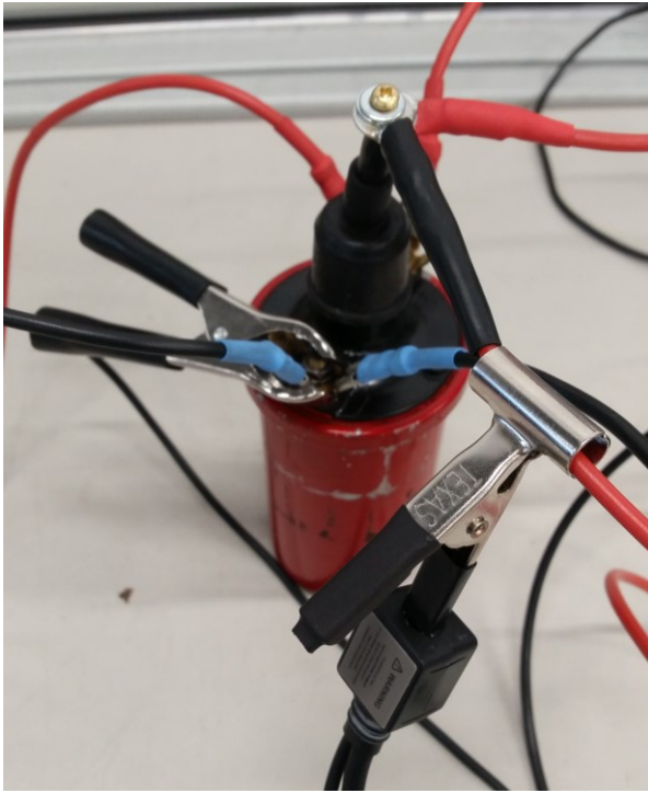
Figure 23. Pico Technology MI074 inductive capacitance probe connected to the secondary side output of the Biltema 1880 ignition coil.
