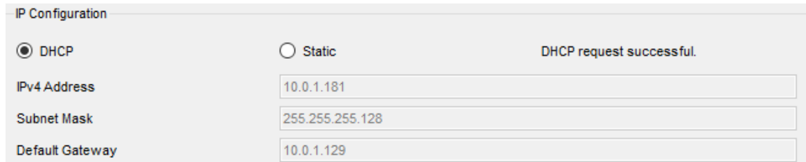
Figure 29 Network information for the end-user network of the second floor backup optical line
