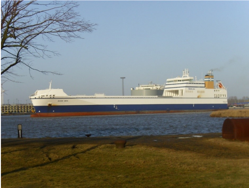
Picture 3 RoRo ship Bore Sea capable of carrying 13 535 DWT or 2863 lane meters
