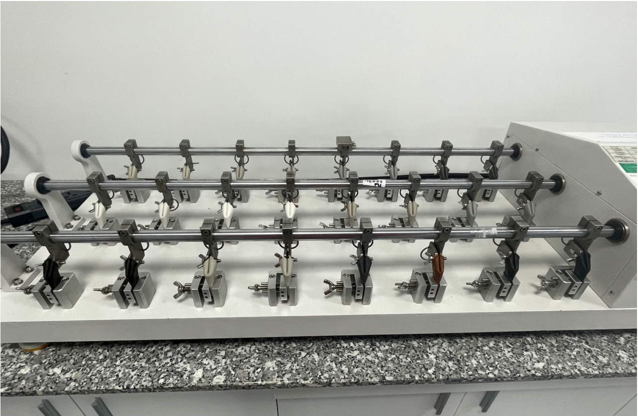
Figure 13. Folding test for leather
