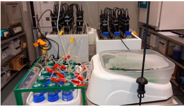
Figur 3. Automatic Methane Potential Test System II (AMPTS II) apparatur. Foto: Viveka Öling-Wärnå.
