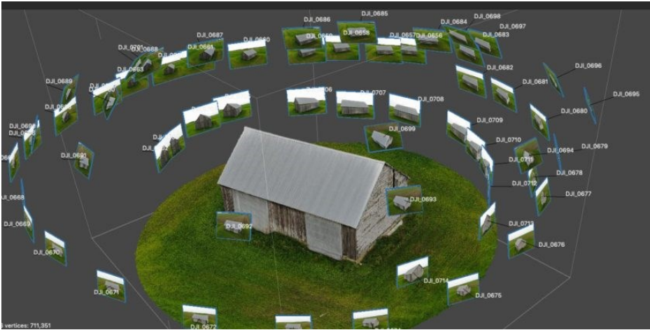
Figure 1. Example of a close-range photogrammetry workflow (Bitfab, n.d.)
