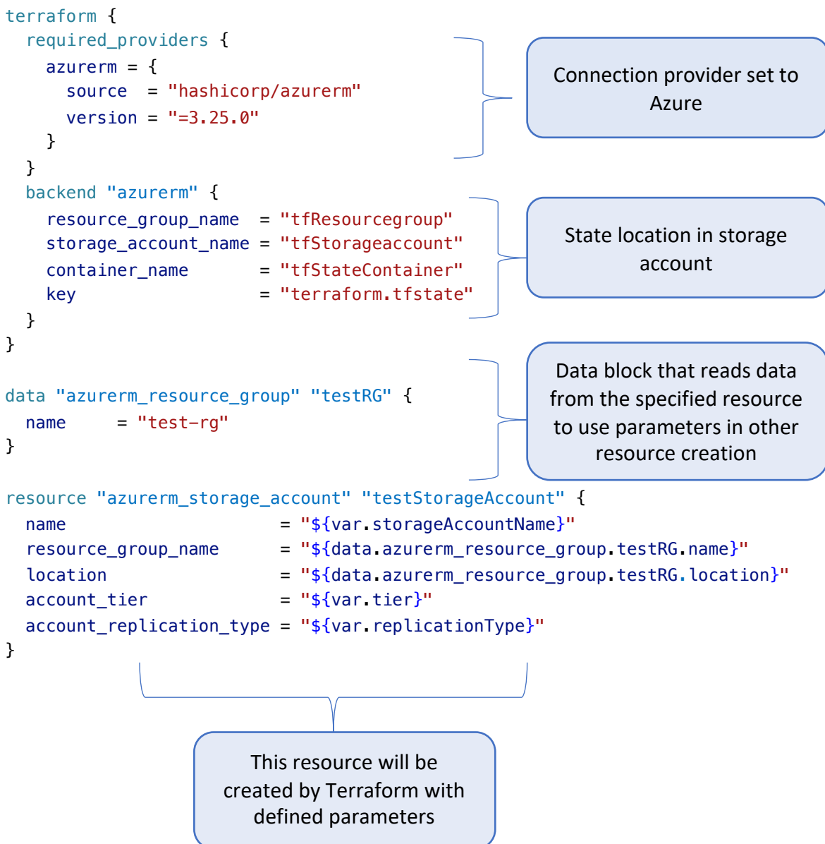
Figure 8 Terraform base structure
