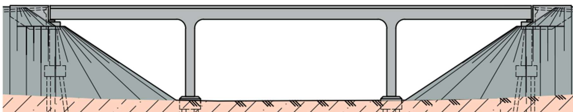
Figure 10. Continuous rigid-frame bridge
