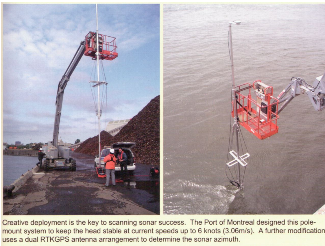
Figure 3.44 Pole-mount Deployment for Imaging and Profiling
