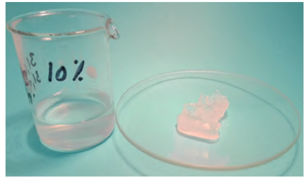
Figure 2. Otto Långvik is interested in developing new materials from the lignocellulosic feedstocks. To the right you see a hydrogel made by copolymerizing methacryl acid with 10% methacryl functionalized galactoglucomannan.
