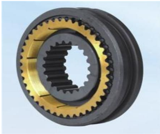
Figure 2.3 The real lock ring synchronizer (Automotive Transmission, 2013, p.1).
